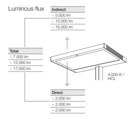
State-of-the-art LEDs provide either symmetrical or asymmetrical light distribution via a light panel. VITAWORK<sup>®</sup> is suitable for complete illumination of larger and more spacious offices. In the development of this range, we have placed special emphasis on energy efficiency (approx. 135 lm/W). Depending on the application, VITAWORK<sup>®</sup> fulfils the requirements of the EN 12464-1 standard and the German workplace ordinance ASR 3.4.
